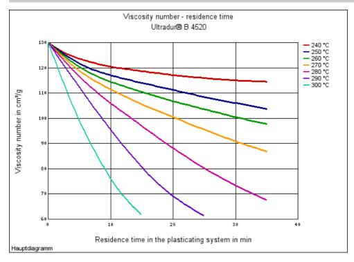
Unnecessarily high melt temperatures and excessively long residence times of the melt in the cylinder and the hot runner can bring about molecular degradation.
